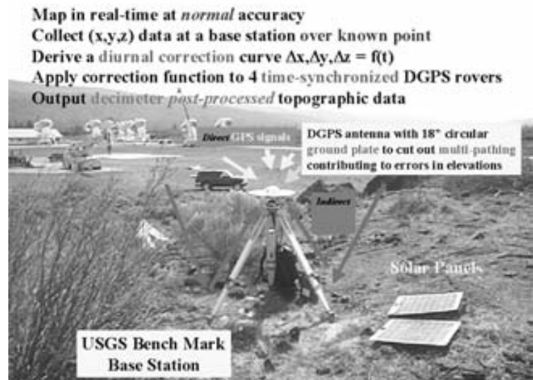
Figure 8. GPS base station set-up showing solar panels for power. Note radio telescopes in the background. Reference point is a permanent USGS survey monument.
