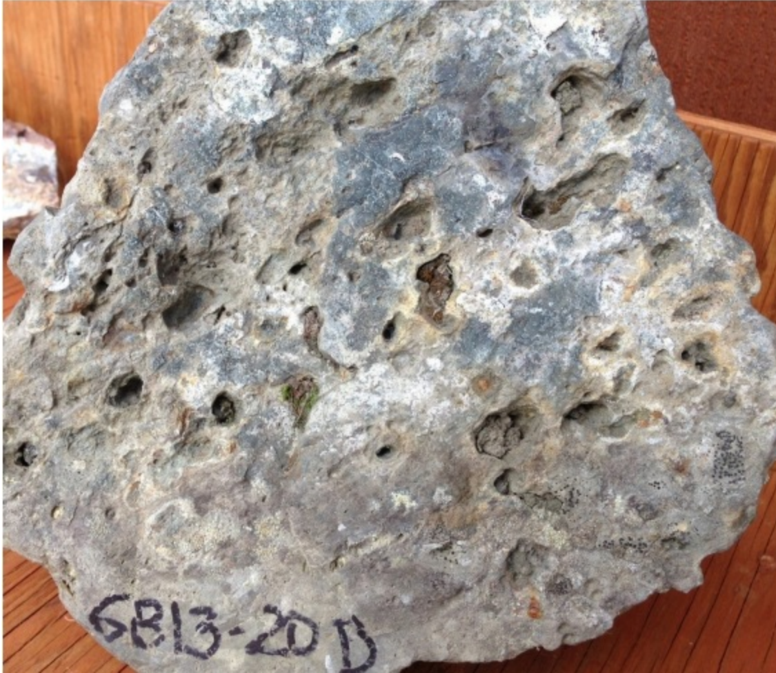
Figure 1. Orbicular wall rock alteration consisting of chlorite and muscovite-lined orbs up to about 1- inch diameter also containing sparse disseminations of chalcopyrite, pyrrhotite, and ilmenite. Sample from the west side of the Clementine anticline along the Indian Creek Road.
